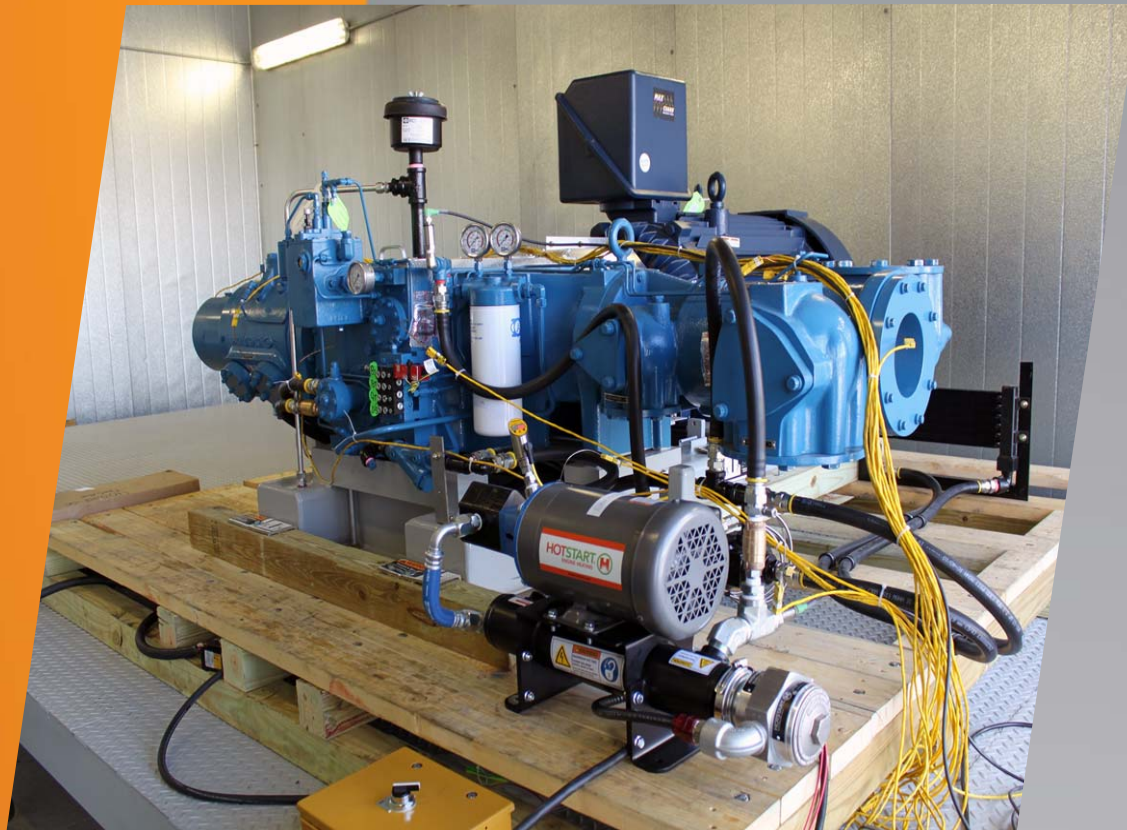
Ariel JPG/2 Cold Room Testing
