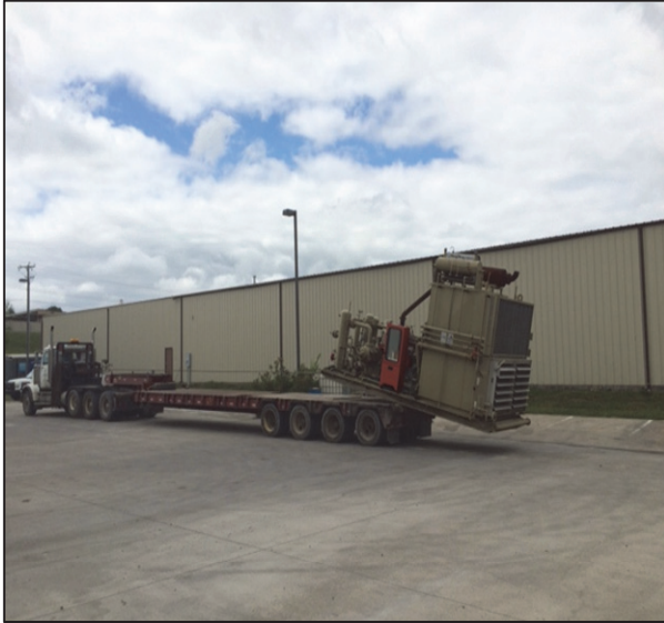
Figure 20: Smaller compressor packages are typically tail-boarded with a winch truck.
