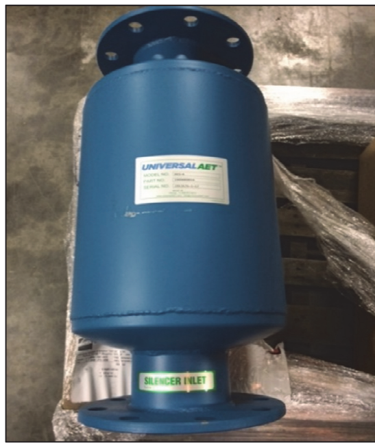
Figure 18: An off-the-shelf silencer for gas exhaust vents, such as PSVs.
