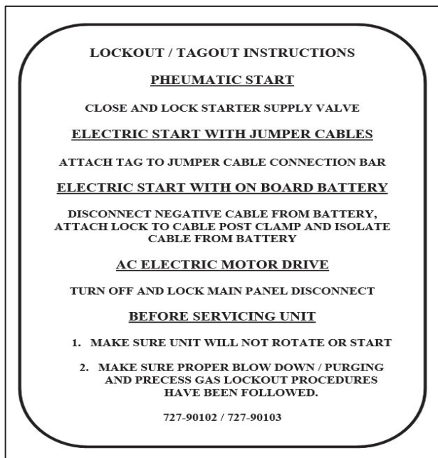
Figure 2: Close-up of the instructions on the decal in the panel door on Figure 1.
