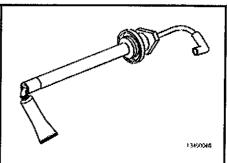
Install the spark plug adapter (2).
