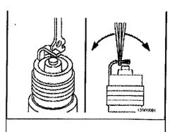
A magnetic spark plug socket can be used to install the spark plug.
